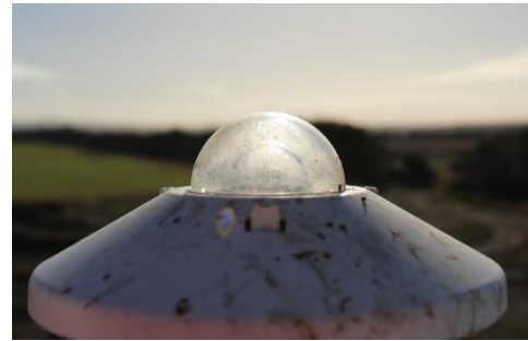
Figure 1 - Heavily soiled pyranometer, accumulated during 7 days without cleaning.
